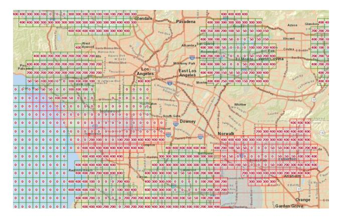
The FAA has forged partnerships with several companies that provide mobile apps providing near real-time processing of airspace authorizations for Part 107 drone operators who fly in controlled airspace. It's part of what's called the Low Altitude Authorization and Notification Capability (**LAANC**) initiative.
